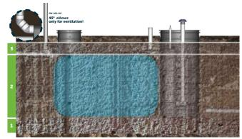
**4** - To finalize the installation, backfill the surface to a height of 20 cm using the excavated topsoil, previously cleared of any stony or sharp elements, then position and secure the covers.
