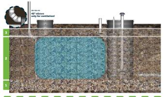
4 - To finalize the installation, backfill the surface to a height of 20 cm using the excavated topsoil, previously cleared of any stony or sharp elements, then position and secure the lids.
