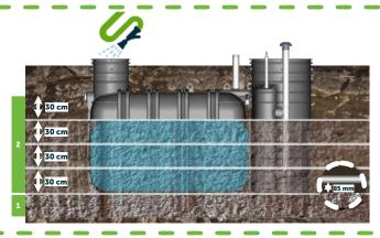
**3** - When the backfill level reaches just below the level of the hydraulic and ventilation connections, make the connections. Backfill to 20 cm under the lids and compact.
