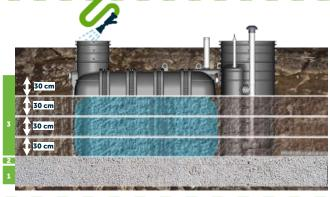
**4** - When the backfill level reaches just below the level of the hydraulic and ventilation connections, make the connections. Backfill to 20 cm under the lids and compact.
