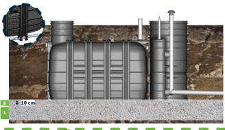
**3 - Backfill in 30 cm increments while simultaneously filling the primary tank with clean water.** Compact **manually** between each slice.
